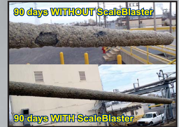
Actual Test Coupons from the PChem Wastewater Treatment Facility in Illinois
