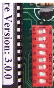
View of the Dip Switch set for normal mode.
