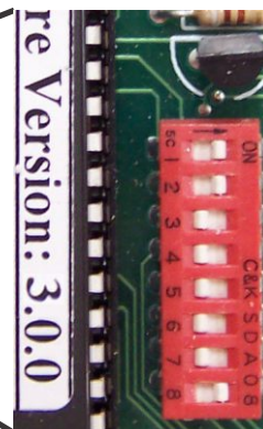
Close up view of the Dip Switch set for calibration mode
