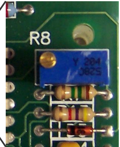
Close up view of potentiometer on slave board
