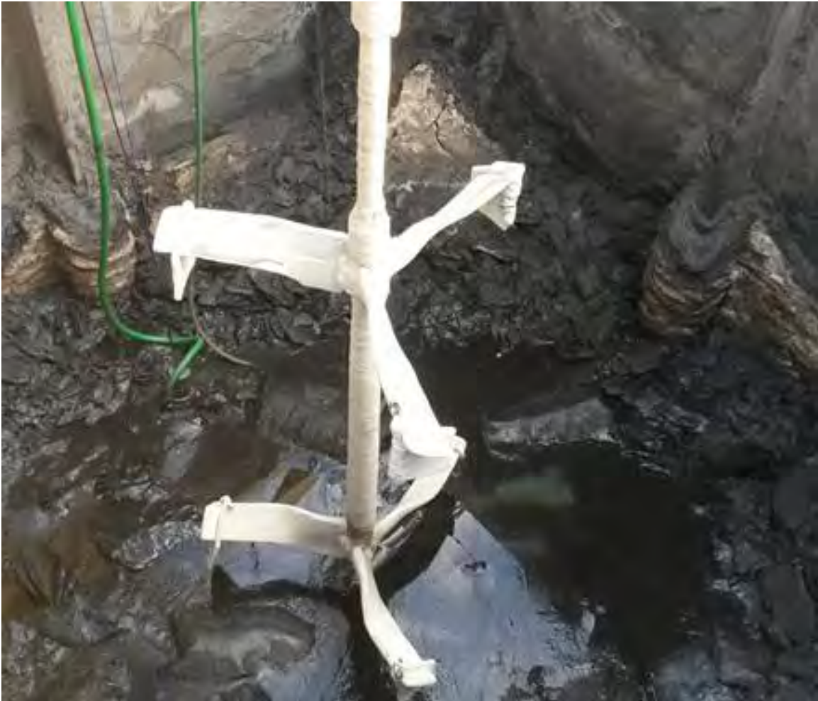
Photo 23: Neutralizer Agitator taken March 27, 2015
